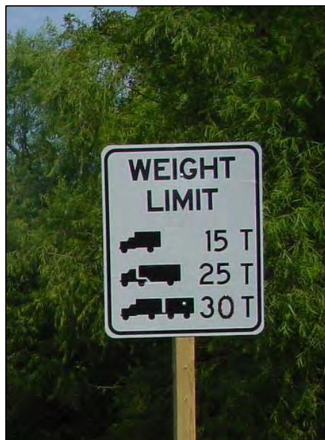
Figure 130. View of MUTCD R12-5 weight limit sign for Bridge Number 15558X.
